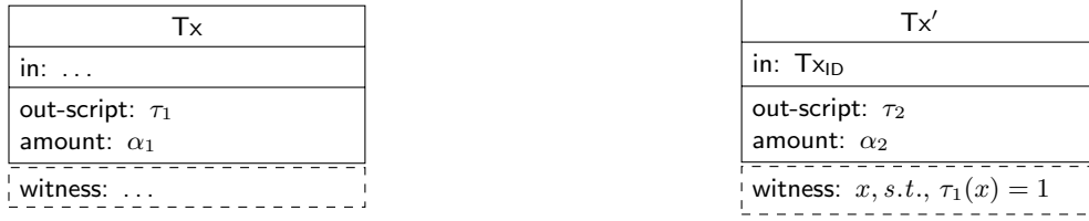
Figure 3: The structure of a transaction in Bitcoin. The transaction Tx' is spending the output \tau_1 of transaction Tx.
