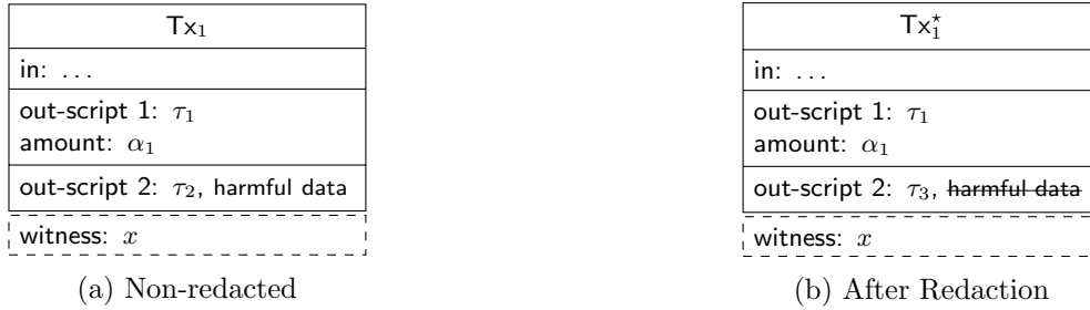
Figure 5: (a) The transaction T_{x_1} contains harmful data, and (b) the candidate transaction T_{x_1}^* contains a copy of all the fields of T_{x_1} , with exception of the harmful data.
